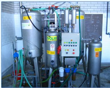
Fig. 1. Biodiesel processor 200, Preseco Oy Finland
